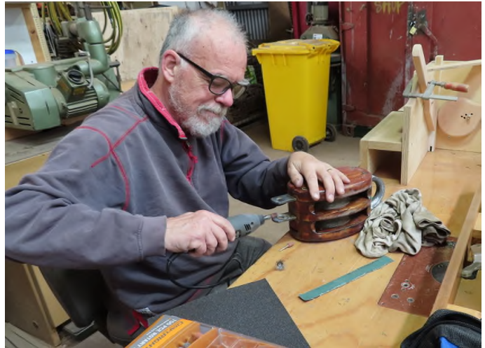
Ian refurbishing block of anchor davit Nov 2021
