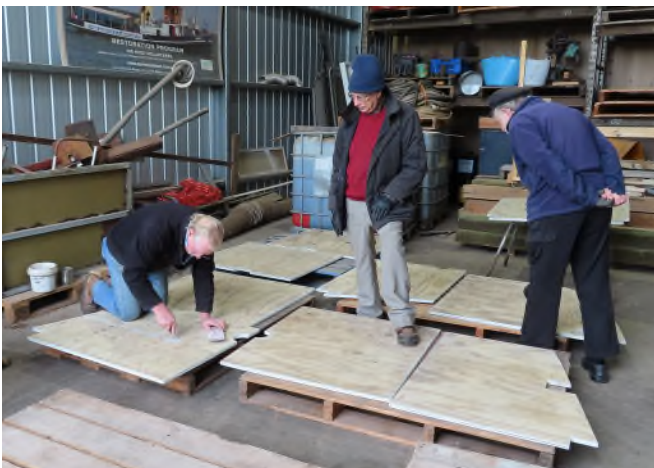
Cutting and preparing galley flooring March 2020
