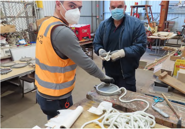
Sabastian and Alex sealing galley portholes, July 2021
