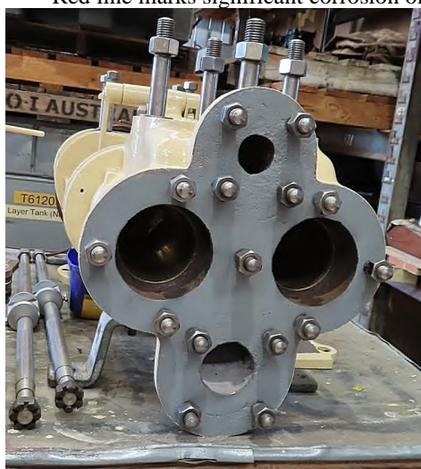
Refurbished GS pump approaching installation July 2021 Note new stainless steel piston rods .
