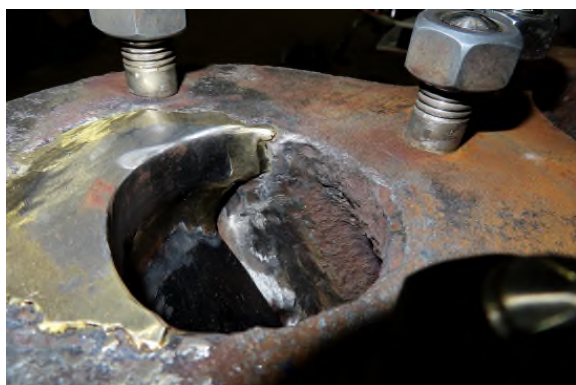
The fix -aluminium bronze welding to cast iron May 2021
