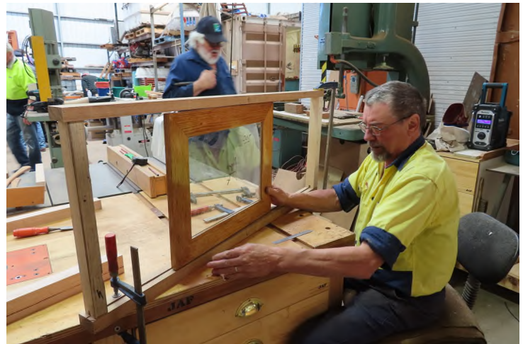
John making sliding door for galley dumb waiter, Dec 2021
