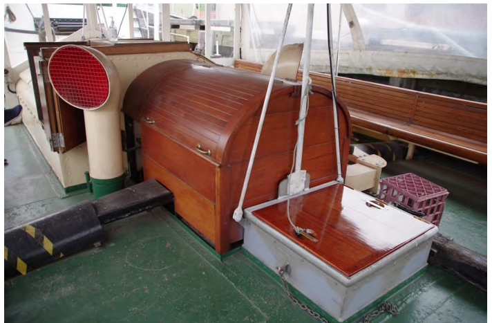
Steering engine cover and generator hatch cover completed
